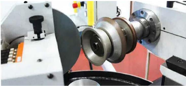
Figure 7: Trueing on an external machine
