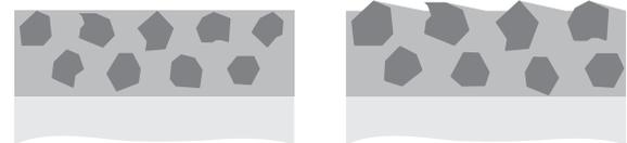
Figure 5: Aim of the sharpening - Creation of grain overhang (micro geometry)
